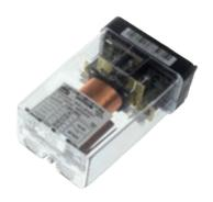
The N.S1-L-24-4.0.4 is a 24 VDC track side safety relay for the signalling railway market. It is a single module plug-in relay with positive mechanical keying, equipped with 4 normally open contacts and 4 normally closed contacts.
