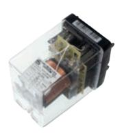
The N.S1-L-24-12.0.8 is a 24 VDC track side safety relay for the signalling railway market. It is a dual module plug-in relay with positive mechanical keying, equipped with 12 normally open contacts and 8 normally closed contacts.
