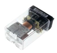
The N.S1-P-24-4.0.4 is a 24 VDC track side safety relay for the signalling railway market. It is a single module plug-in relay with positive mechanical keying, equipped with 4 normally open contacts and 4 normally closed contacts.
